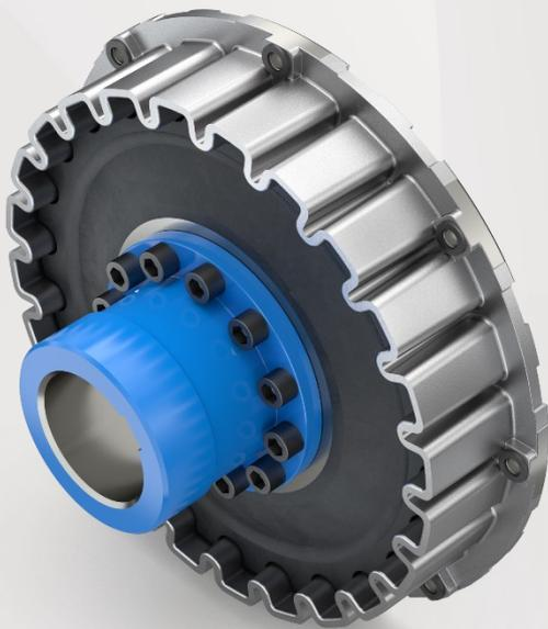
Another key factor in the success of this coupling design is the selection of different rubber compounds which are manufactured in-house by REICH. These can be chosen to provide the correct torsional characteristics for the diversity of applications which may be encountered in the field and meet ambient operating temperatures which can be from -70°C up to +130°C in extreme cases.
